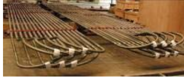
Cracking Tubes for Ethylene
