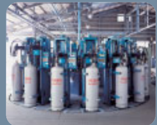
LPG FILLING SYSTEM
