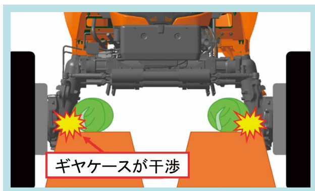
図6 ギヤケースと作物の干渉 Fig. 6 Interference Between the Gear Case and the Crop
