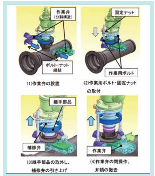
図10 交換工法の手順 Fig. 10 Replacement Method Procedure
