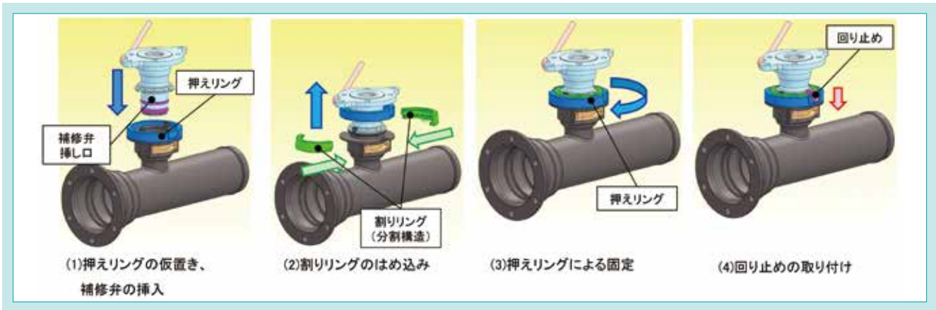
図6 接合手順 Fig. 6 Procedure for Jointing
