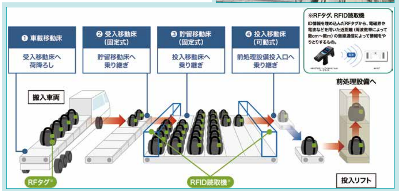
図5 受入ヤードの自動化 Fig. 5 Receiving Yard Automation
