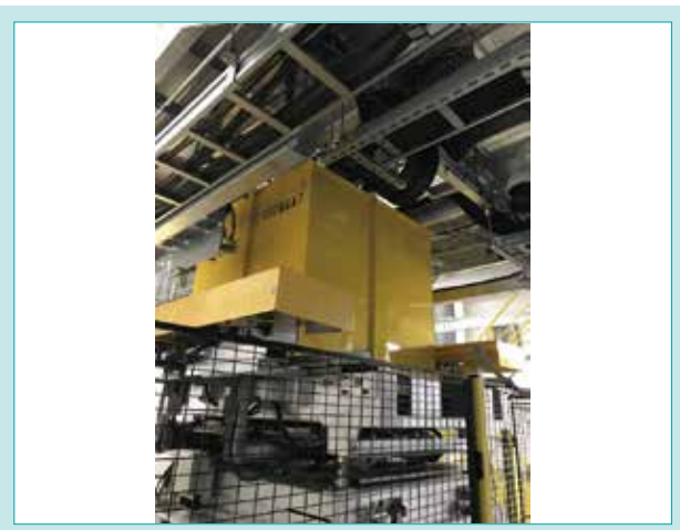
図6 鋼製角形容器への充填 Fig. 6 Filling a Steel Square Container
