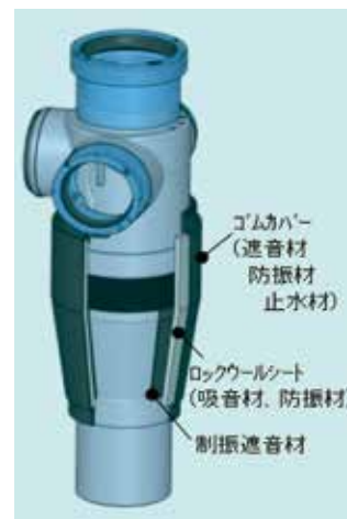
図3 遮音材の構成 Fig. 3 Composition of Sound Insulation Material
