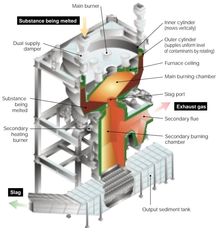
Structure and operation of the melting furnace
