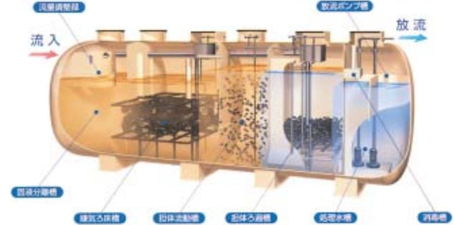
We realized a high efficient treatment by a fluidizing-carriers-filtration method.
