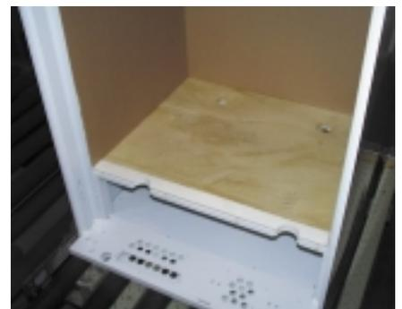
Board-type heat insulating material
