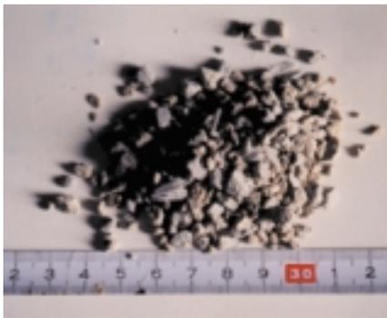
Photo 3. Recycled material from FW pipes (mortar layer)
