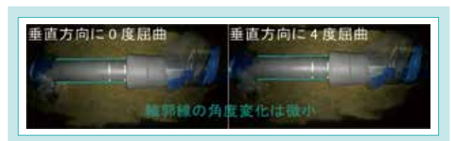
図7 継手屈曲角度の確認 Fig. 7 Checking Joint Deflection Angles
