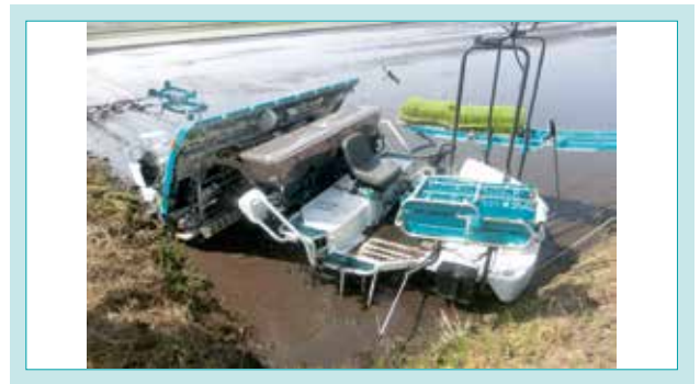
図2 走行不能に陥った田植機 Fig. 2 Rice Transplanter that has Become Bogged Down
