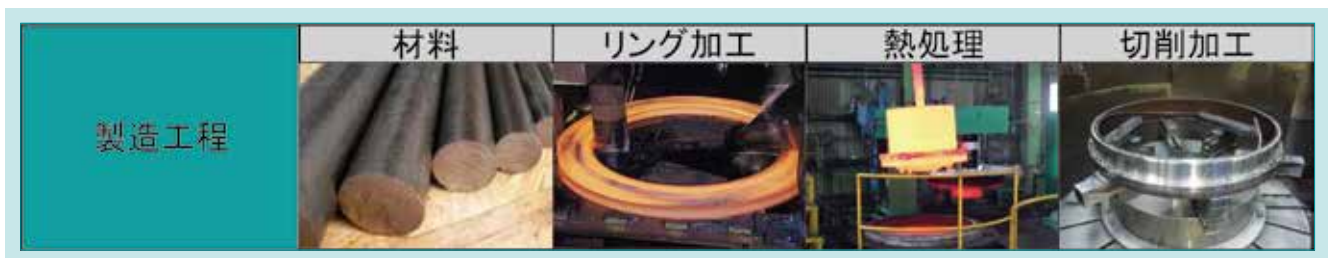
図2 機械式継手の製造工程 Fig. 2 Manufacturing Process of a Mechanical Joint
