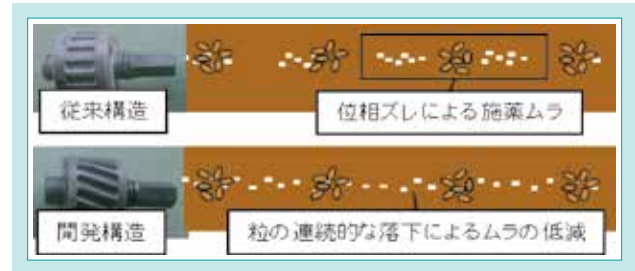
図 12 施薬ムラの改善 Fig. 12 Continuous Falling of Agrochemicals
