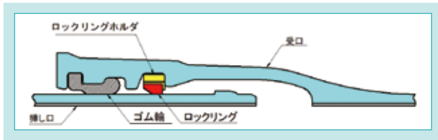
図1 GENEXの継手構造 Fig. 1 Joint Structure of GENEX
