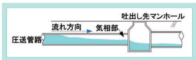
図6 腐食危険箇所(管路吐出し先) Fig. 6 Flow Condition Around Manhole
