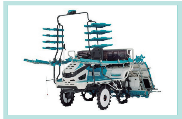
図2 直進キープ機能付田植機「EP8D-GS」(8条) Fig. 2 Rice-transplanter "EP8D-GS" with Automatic steering (8 rows)
