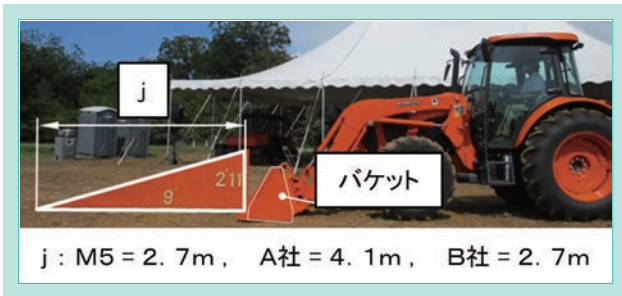
図7 ボンネット前方の視界性比較 Fig. 7 Comparison with Competition of Visibility in Front of Bonnet
