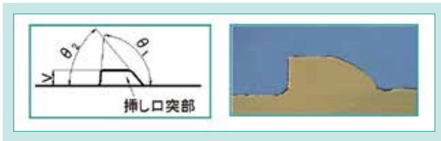
図 13 挿し口突部の断面形状 Fig. 13 Cross-section Shape of Spigot Projection
