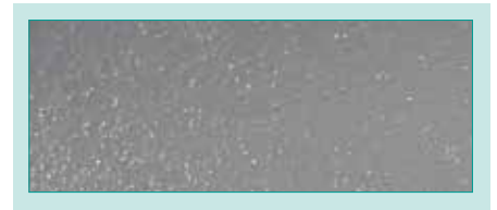
図 17 珪砂混合エポキシ樹脂粉体内面塗装 Fig. 17 Epoxy Resin Powder Coating Mixed with Silica Sand
